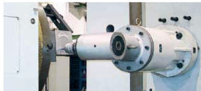
40 or 60 tool Automatic Tool Changer
